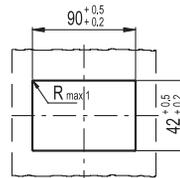
Drilling template for battery case
