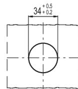
(remove all drilling burrs before fitting the display / battery case)
