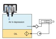
When in the reservoir a depression around 0.030 bar is produced, a flux of air entering the reservoir through the suction valve takes place.
