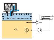
When in the reservoir an over pressure exceeding 0.350 (or 0.700) bar is produced, a flux of air is discharged through the safety valve.
