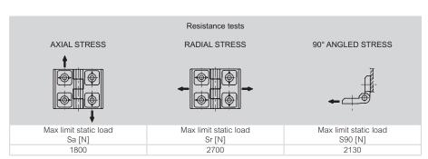
The max static load is the value above which the material may break thus prejudicing the hinge functionality. Obviously, a suitable factor, according to the importance and the safety level of the specific application must be applied to this value.
